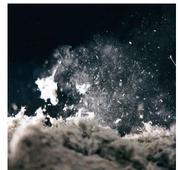
Airborne asbestos fibres released from pipe lagging
